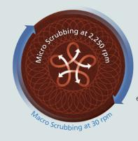
Patented REV™ random orbital scrubbing technology with high-speed, ¼-inch micro scrubbing and rotational, low-speed macro scrubbing attacks dirt from multiple directions for superior cleaning effectiveness.
