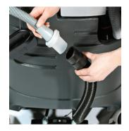
The squeegee hose eliminates the need for a drain hose and also helps rinse the recovery tank clean and reduces dirt build-up.
