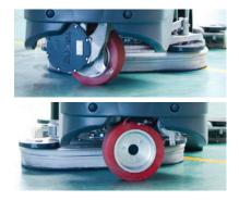
The SafetyGlide™ Deck automatically moves in line with the path of the rear squeegee when the steering wheel turns.
